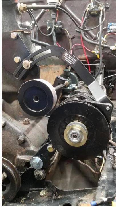
Side-mount water pump and alternator pulleys
