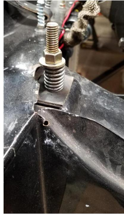
Radiator bolt assembly held in place w/magnet
